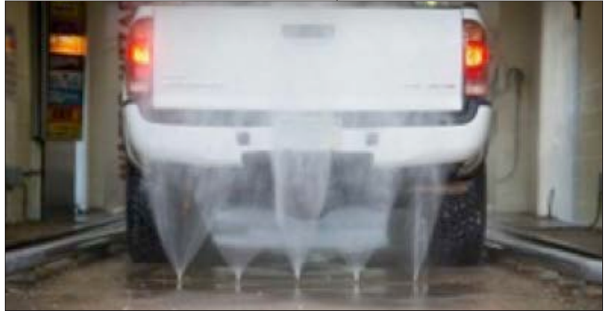
An automatic car wash with undercarriage spray nozzles. Image: Wash Me Car Washes
