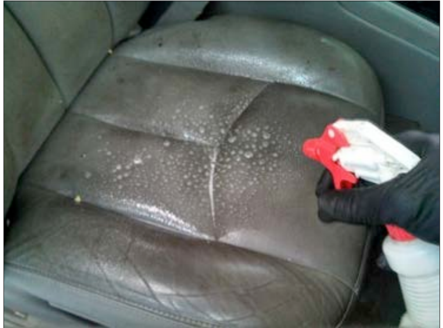
Applying cleaning solution to a leather car seat. Image: Auto Detail Doctor
