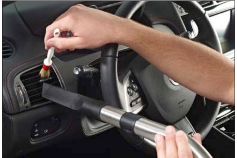
A detailing brush helps remove dust from ventilation ducts and other hard-to-reach areas.
