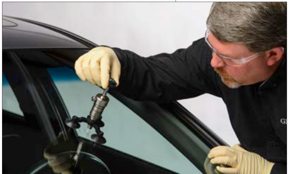
Chip repair can be a cost-effective alternative to windshield replacement. Image: GlasWeld
